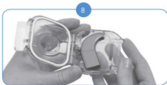
The Naída CI should fit tightly to the back wall of the AquaCase and lie flat against the bottom surface.
