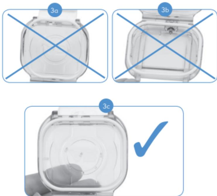
To insert the new O-Ring, place a portion of the new O-Ring in the AquaCase mounting groove on the case. Take care to match the rectangular shape of the O-Ring correctly with the rectangular shaped AquaCase.
