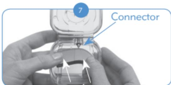
Line up the processor headpiece cable connector (located on the back spine of the Naída CI below the Program Button) with the cable connector located inside of the AquaCase. Slide the Naída CI into the AquaCase until the connection is made.
